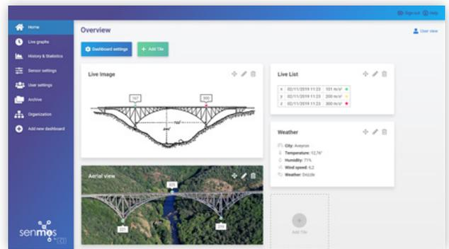
Dashboards to give quick overviews of the structure. With features such as: Images with live values, graphs with live data, tables with sensor values, and much more.
